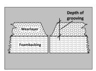
The grooving depth of seams must never be deeper than ¾ of the thickness of the homogenous wearlayer.
