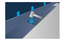
This method is then used to install all of the other rows. Make sure that the end joints are offset by at least 30 cm in the individual rows in order to achieve the best installation. To install the last row, the distance between the wall and the row installed is measured and transferred to the panel. The last row installed should be as close to half a panel's width as possible. Remember the 6 mm wide expansion joint.
