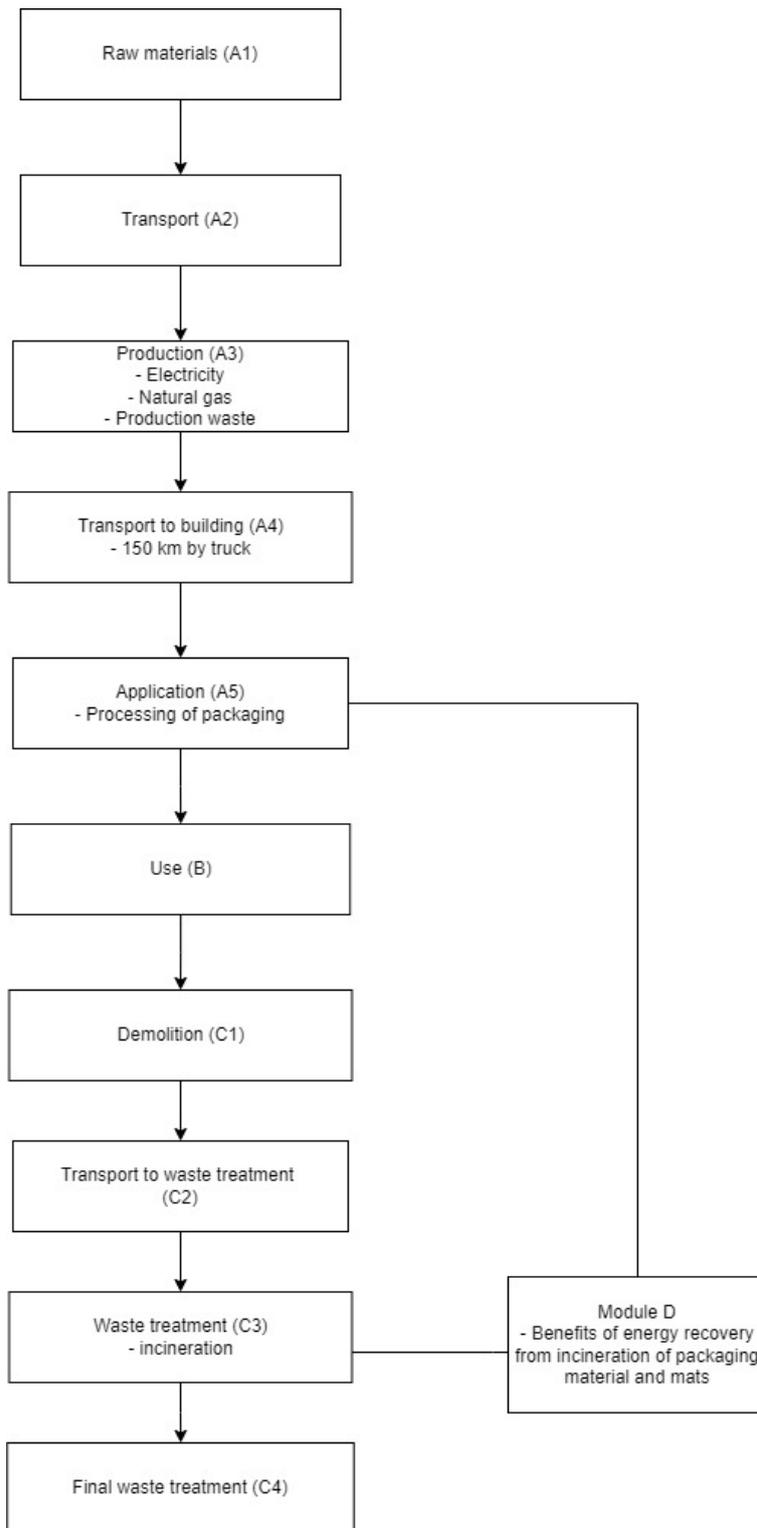
Figure: LCA process diagram according to EN 15804 (7.2.1)
